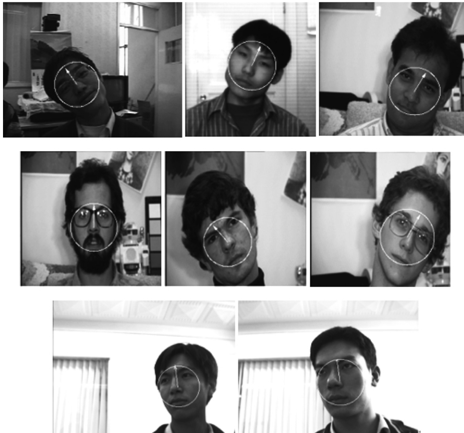
Fig. 5. Some experimental results of the rotated face detection (the white circle is the circle mask used in calculating the histogram and the arrow refers to the orientation of the principal axis obtained by our algorithm).
